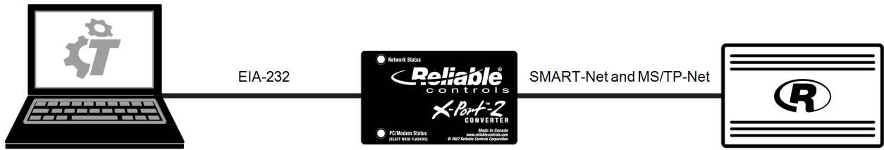
Figure 16: Computer connection to the controller's SMART-Net and MS/TP ports using the X-Port-2
